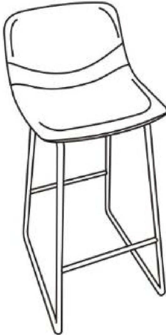
**Important Note – Before finally tightening the bolts, place the assembled stool upright on a level surface and sit carefully on the stool to ensure the chair legs are aligned and level. Then tighten all bolts and your stool is ready for use.**
