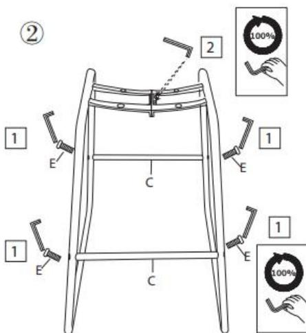
Join Connector bars (C) with Bolts(E) By using Allen Key (D) Screw to 100%, Tighten the Step ① to 100%
