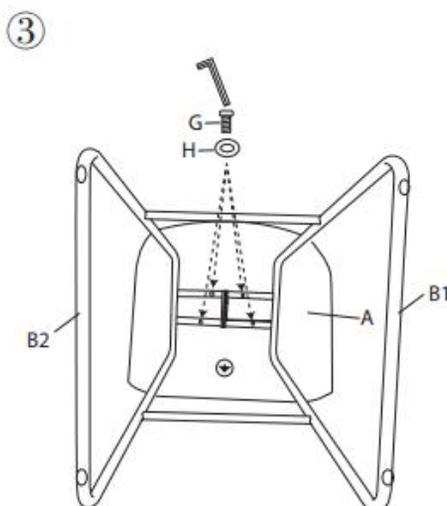
Attach Stool Seat (A) to constructed Base with Bolt (G) and Spacer (H) Using Allen Key (D)
